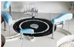
Reaction Tray 37±0.1°C, real-time monitor.
