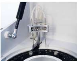
Washing Probe Independent 2-step washing system.
