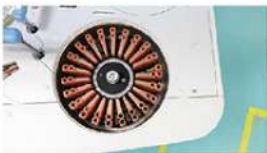
Reagent Tray 2~8°C cooling for 24 hours
