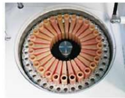
Reagent Tray Refrigerated tray with independent switch.
