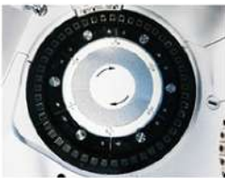
Reaction Tray 37±0.1°C, real-time monitor.
