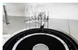
Washing Probe Independent 7-step washing system.
