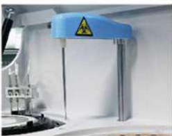
Sample Needle Liquid level sensor function. Anti-collision function. Reagent volume real-time detection.
