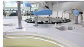
Mixer Probe Dual mixer, auto frequency adjustment
