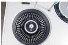
Reaction Tray 37±0.1°C, real-time monitor.
