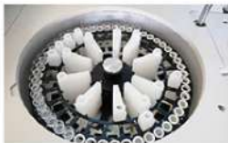
Reagent Tray 2~8°C cooling for 24 hours.
