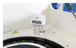
Washing Probe Independent 4-step washing system.
