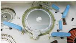
Reaction Tray 37±0.1°C, water bath
