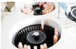
Reagent Tray 2~8°C cooling for 24 hours.
